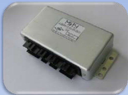
Informational control module for the bus MAZ-231
